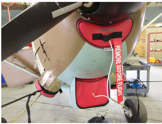
Siai Marchetti 1019 Engine Plugs, Prop Tie-Exhaust Covers
