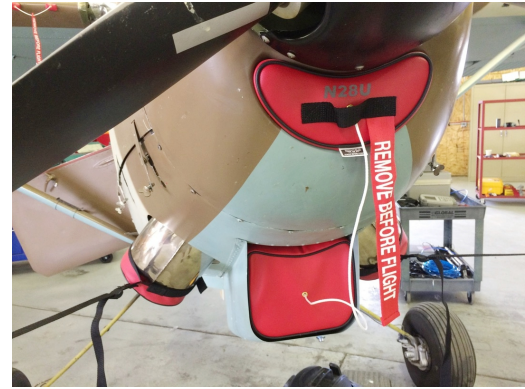
Siai Marchetti 1019 Engine Plugs, Prop Tie-Exhaust Covers
