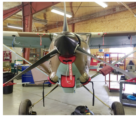
Siai Marchetti 1019 Engine Plugs, Prop Tie-Exhaust Covers
