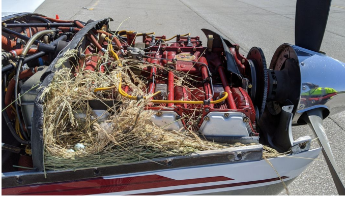
ENGINE PLUGS PREVENT BIRD NEST FOD. Piper Saratoga Engine Cowling Bird's Nest Aeronca 7AC Engine Inlet Plugs
