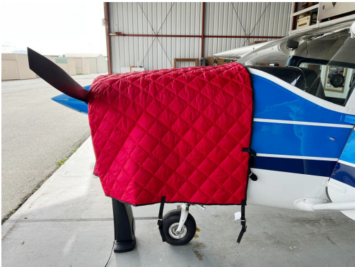
Insulated Hangar Blanket on Cessna 182
