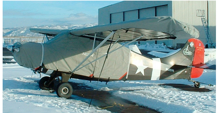
Extended Canopy Cover, Engine & Wing Covers
