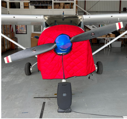
Insulated Hangar Blanket on Cessna 182
