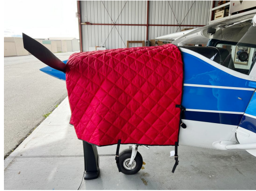
Insulated Hangar Blanket on Cessna 182
