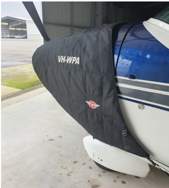
Cessna 182 Insulated Engine Cover, fully enclosed
