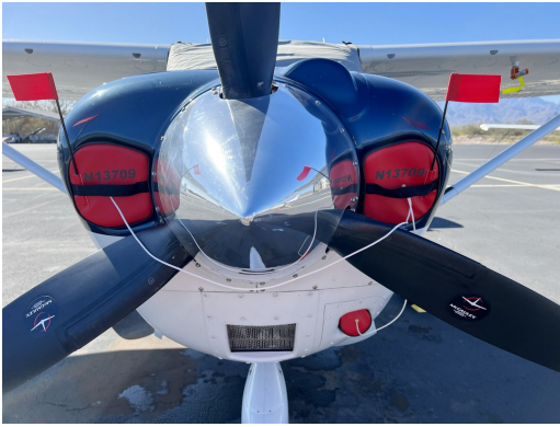
Cessna 206 Engine Inlet & Oil Cooler Plugs ENGINE PLUGS PREVENT BIRD NEST FOD. Piper Saratoga Engine Cowling Bird's Nest
