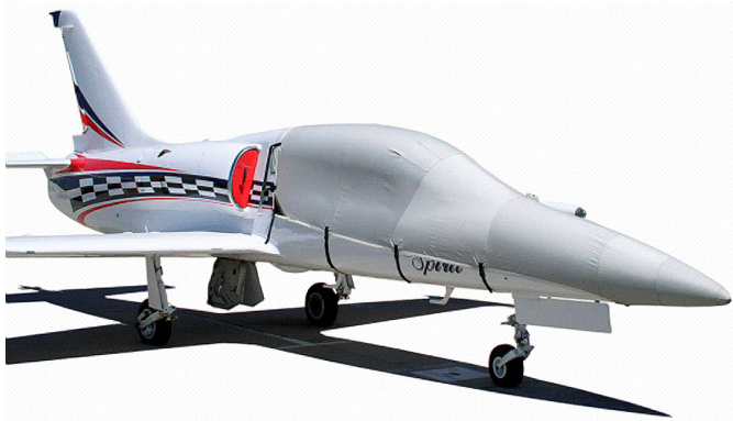
L39 Canopy/Nose Cover & Intake Plugs
