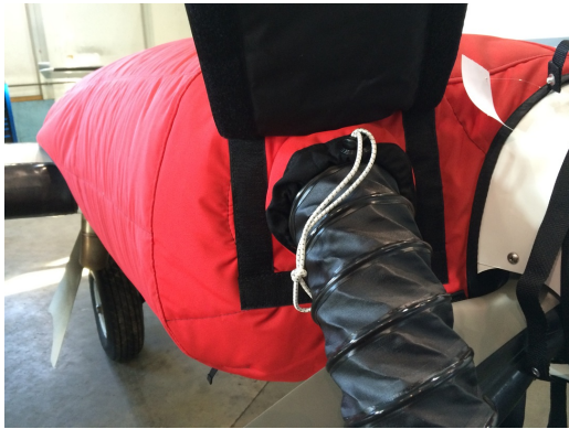
Cessna 402 Insulated Engine Cover with Heater
