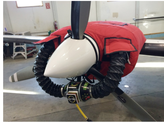
Cessna 402 Insulated Engine Cover with Heater
