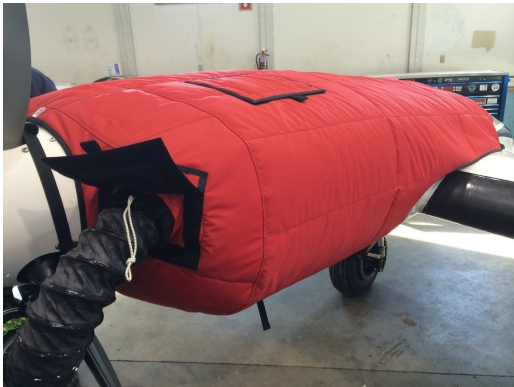
Cessna 402 Insulated Engine Cover with Heater
