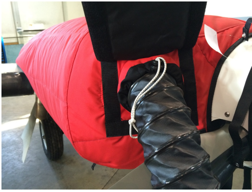
Cessna 402 Insulated Engine Cover with Heater
