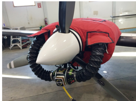
Cessna 402 Insulated Engine Cover with Heater
