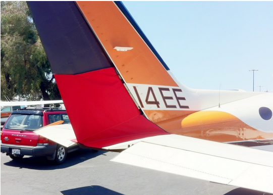
Cessna 414 Rudder Openings Cover (bird barrier)
