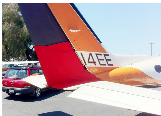
Cessna 414 Rudder Openings Cover (bird barrier)
