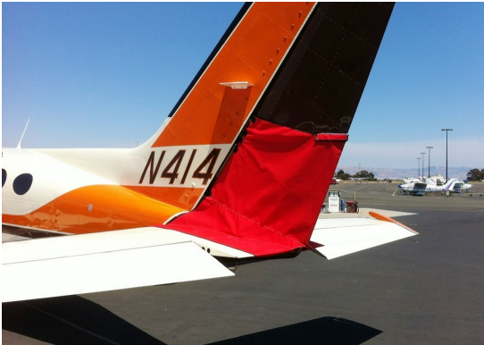
Cessna 414 Rudder Openings Cover (bird barrier)
