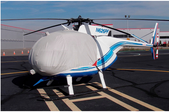
MD500C Bubble Cover with Wire Strike detail
