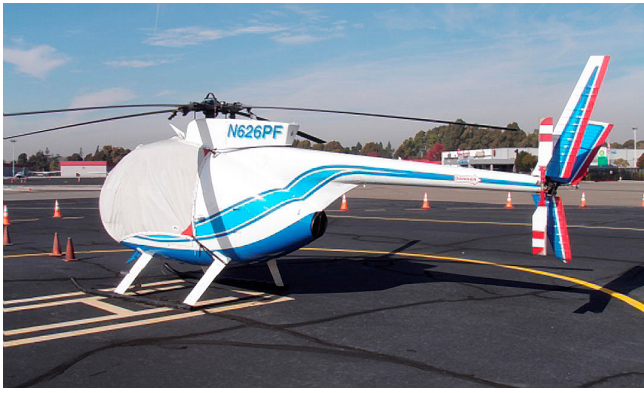
MD500C Bubble Cover with Wire Strike detail
