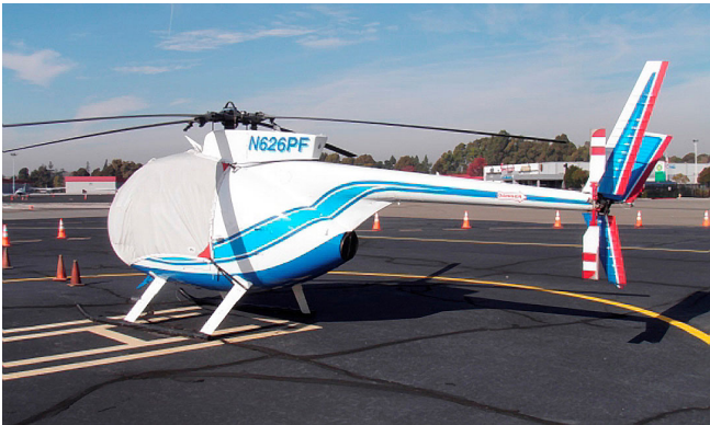
MD500C Bubble Cover with Wire Strike detail
