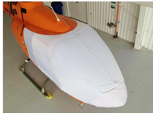
Bell 505 Bubble Cover, test fit cover.
