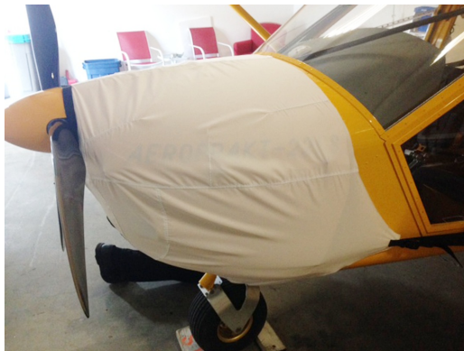
A-22 Engine Cover, test fit
