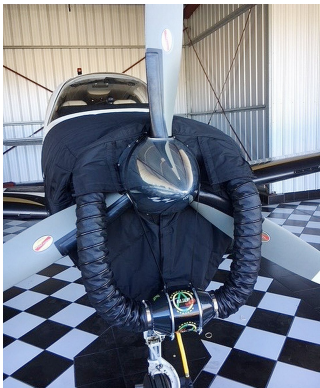
Beech Bonanza 36 Models Insulated Engine Cover
