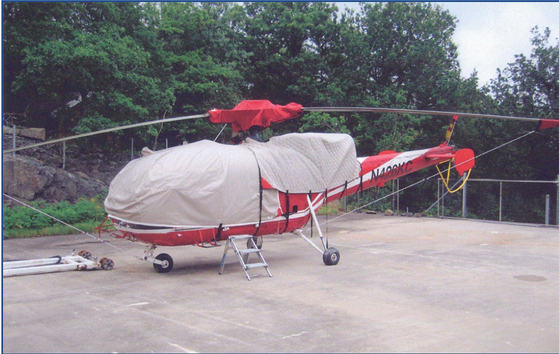
Alouette III Bubble, Rotor Hub &amp; Engine Covers, Blade Tie-Downs
