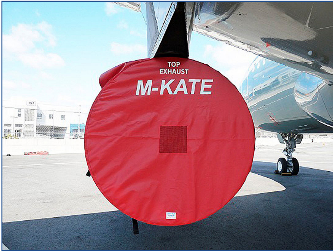
Airbus A319 Intake/Exhaust Covers set, IAE V2500
