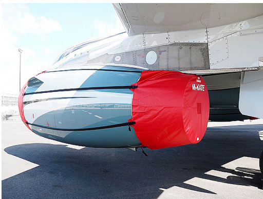
Airbus A319 Intake/Exhaust Covers set, IAE V2500
