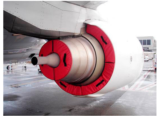
Boeing 737 Bypass and Exhaust Plugs
