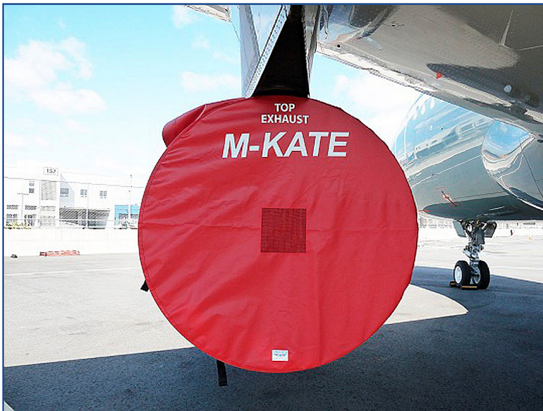
Airbus A319 Intake/Exhaust Covers set, IAE V2500
