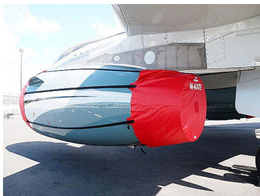
Airbus A319 Intake/Exhaust Covers set, IAE V2500
