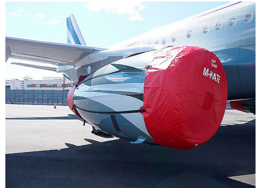
Airbus A319 Intake/Exhaust Covers set, IAE V2500
