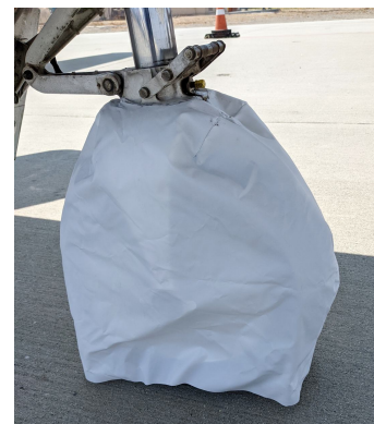
CJ1 Nose Gear Tire Cover, test fit
