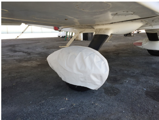
Grumman AA5 Main Wheelpant Cover, test fit
