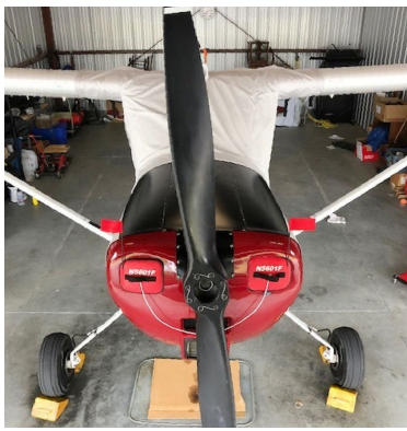
Cessna Bird Dog, L-19, O-1, 305 Engine Inlet Plugs ENGINE PLUGS PREVENT BIRD NEST FOD. Piper Saratoga Engine Cowling Bird's Nest
