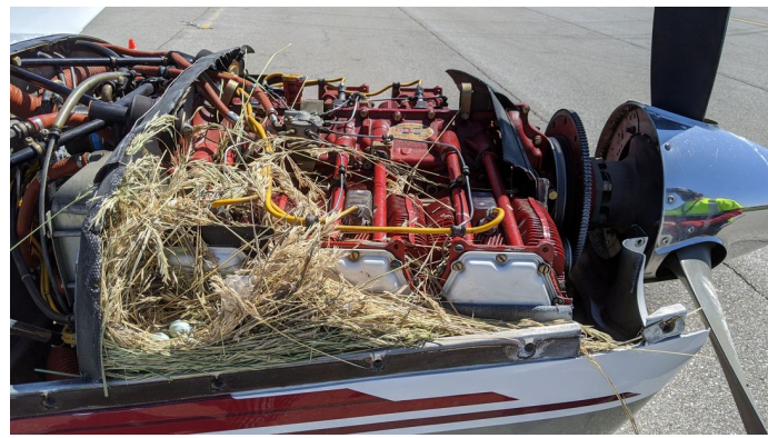
Cessna Bird Dog, L-19, O-1, 305 Engine Inlet Plugs ENGINE PLUGS PREVENT BIRD NEST FOD. Piper Saratoga Engine Cowling Bird's Nest
