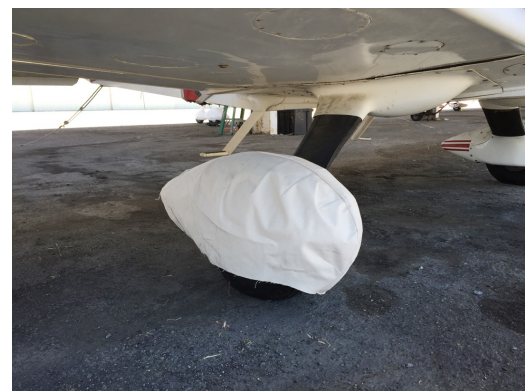
Grumman AA5 Main Wheelpant Cover, test fit
