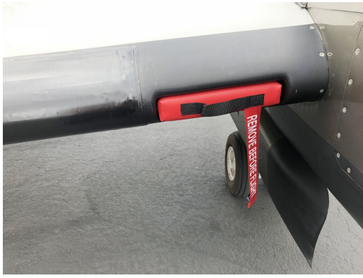
Beech King Air Heat Exchanger Inlet Plug
