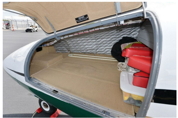
Beech Duke Engine Inlet Plugs stowed in the nose.
