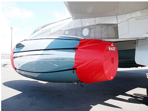
Airbus A319 Intake/Exhaust Covers set, IAE V2500
