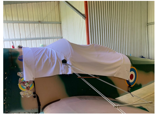
Bowers Flybaby Canopy Cover, test fit design
