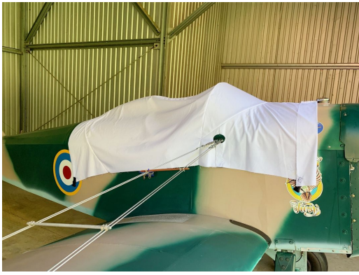
Bowers Flybaby Canopy Cover, test fit design
