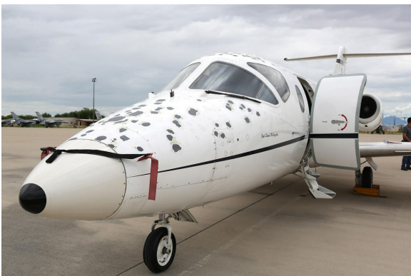
Raytheon Beechjet Hail Damage, and Pitot Covers
