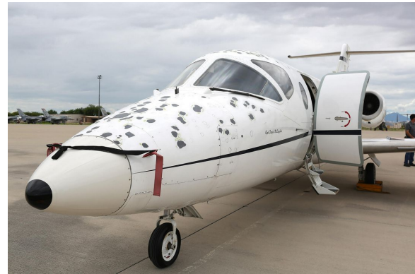
Raytheon Beechjet Hail Damage, and Pitot Covers
