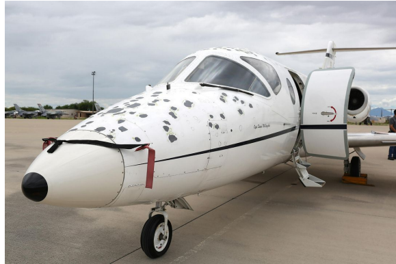
Raytheon Beechjet Hail Damage, and Pitot Covers
