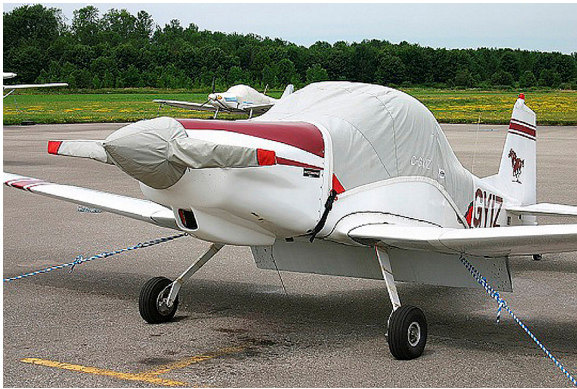
Bushby Mustang Canopy cover and Propellor/Spinner cover
