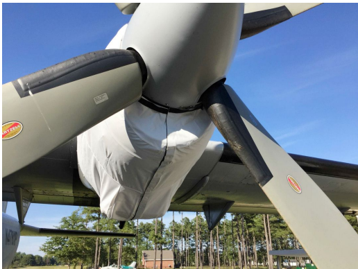
Casa 212 Engine Cover, test fit cover
