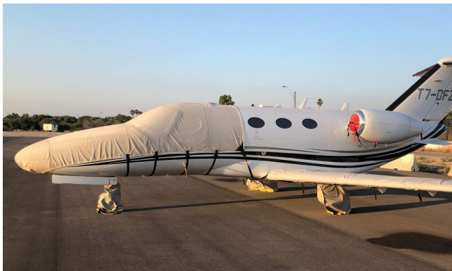
Cessna 510 Mustang Cockpit/Nose Cover, Engine Inlet Plugs
