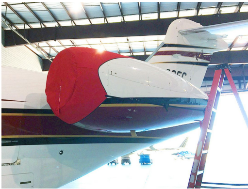
Canadair Challenger 300 Intake/Exhaust Covers, 3-Strap Type Intake/Exhaust Covers, 3-Strap Type. Successfully installed by two crew, one ladder.
