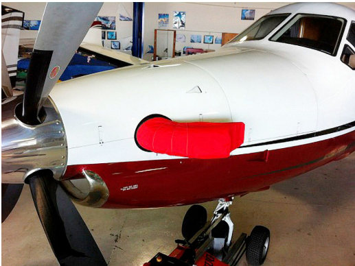
King Air 350 Canopy/Nose Cover, Engine Covers Pilatus PC-12 Exhaust Cover, Fully Enclosed, for protection against corrosion.
