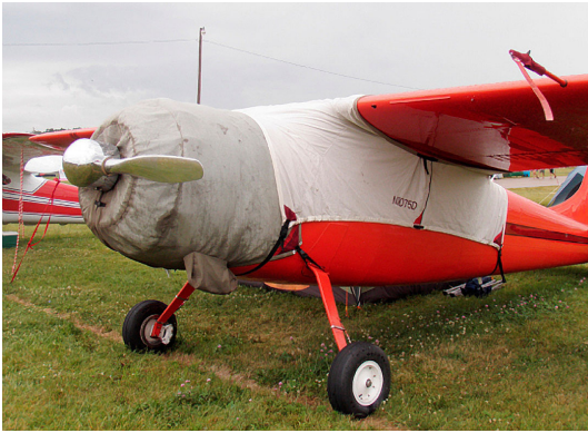
Cessna 195 Over-Top Canopy Cover & Engine Cover
