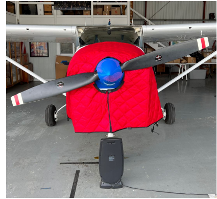
Insulated Hangar Blanket on Cessna 182
