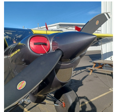
ENGINE PLUGS PREVENT BIRD NEST FOD. Piper Saratoga Engine Cowling Bird's Nest CubCrafters FX-3 Engine Inlet Plugs
