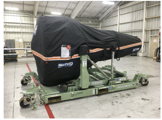
CFM56-5B Off Link Cover, fully enclosed
