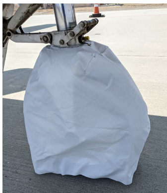
CJ1 Nose Gear Tire Cover, test fit
