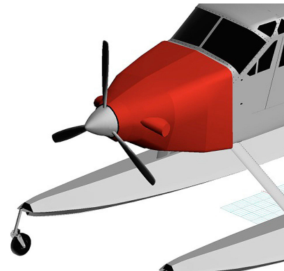
Turbo Beaver Insulated Engine Cover, 3D model
