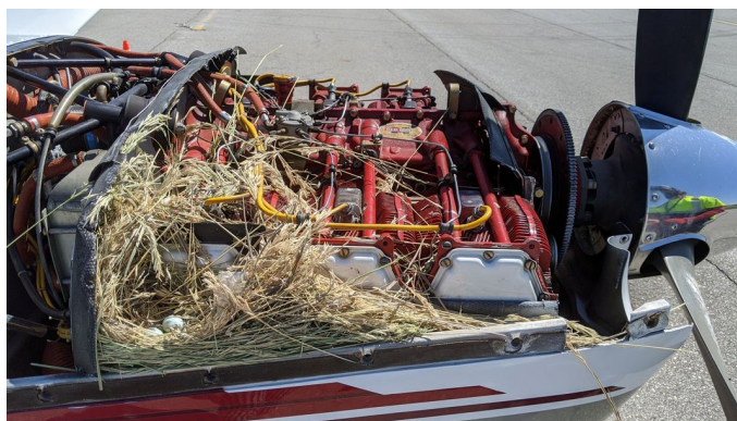
Diamond DA-20-C1 Engine Inlet Plugs ENGINE PLUGS PREVENT BIRD NEST FOD. Piper Saratoga Engine Cowling Bird's Nest
