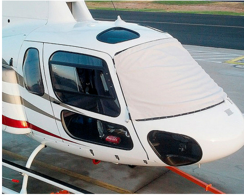
AS350 Windshield Cover, pinches in door jambs
