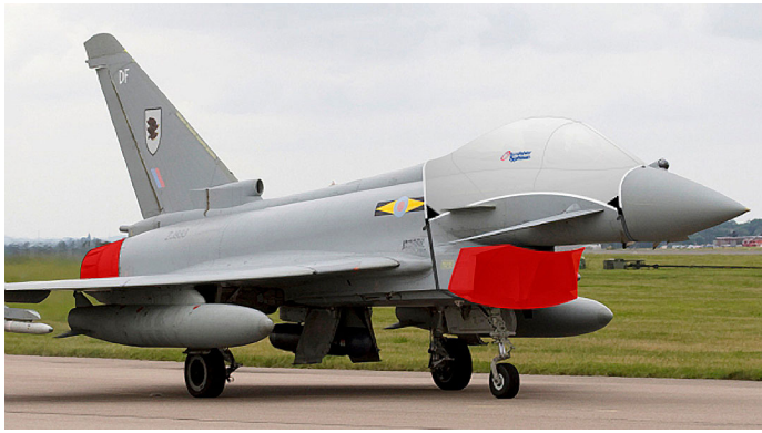
EF-2000 Canopy, Engine Inlet & Exhaust Covers (illustration)
