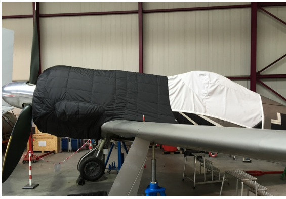
Focke Wulf 190 Canopy Cover & Insulated Engine Cover
