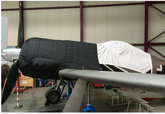
Focke Wulf 190 Canopy Cover & Insulated Engine Cover
