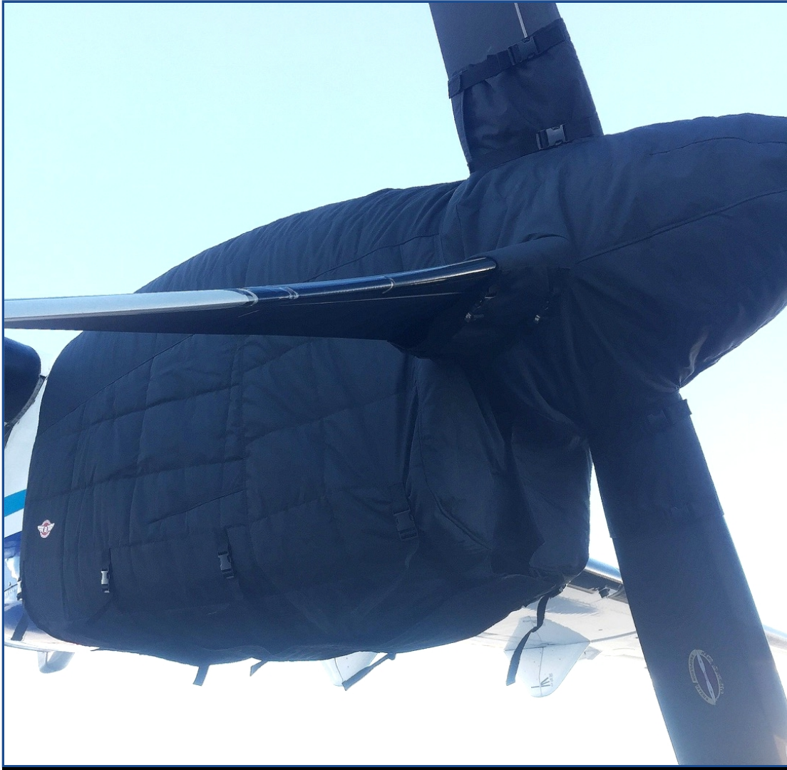
ATR-72-202 Insulated Engine & Prop Hub Covers
