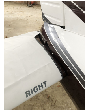
Piper PA-28 Horizontal Stabilizer Cover
