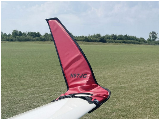
Schempp-Hirth Ventus-2B winglet/wingtip pads
