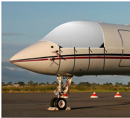
G-V Cockpit/Windshield Cover (Illustration)
