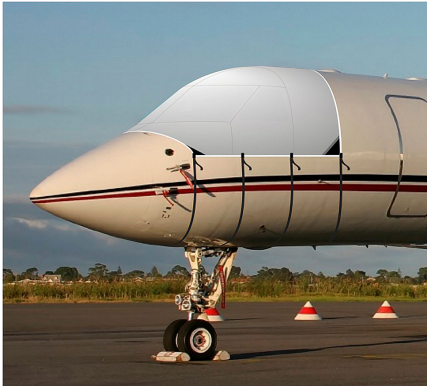
G-V Cockpit/Windshield Cover (Illustration)
