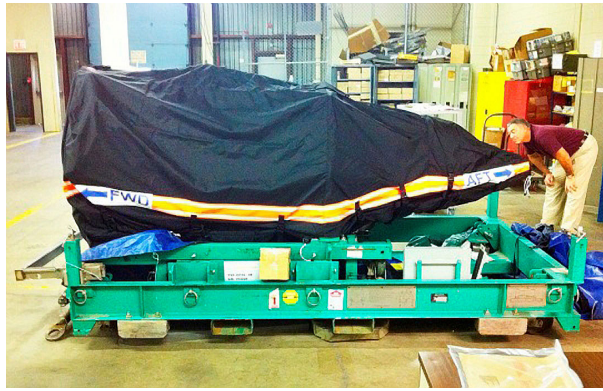
GE CF-34 QEC Engine Long-term Storage/Transport Cover "Bag"
