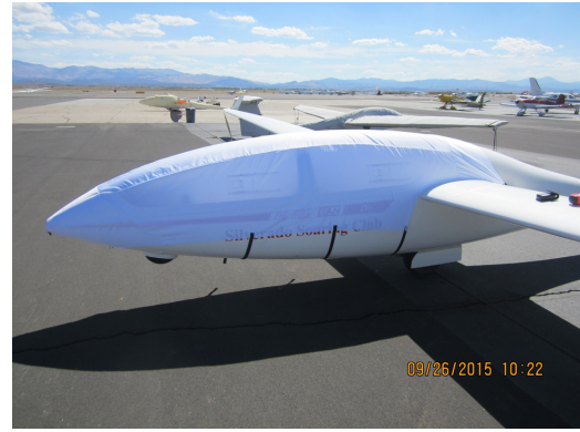
DG-505 Canopy/Nose Cover (test fit cover)
