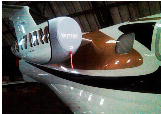
Phenom 100 Intake/Exhaust Cover, "Bikini" Type
